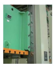
• The SAG slide is guided with 8 sided gibs and adjusted with eccentric bolts.
